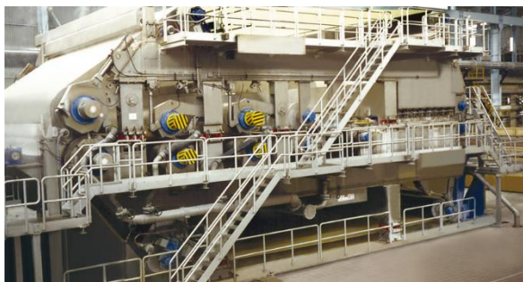
ANDRITZ Twin Wire Press for pulp dewatering
